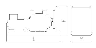
Standard Configuration (open type with base fuel tank)
