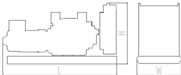
**Standard Configuration (open type with base fuel tank)**
